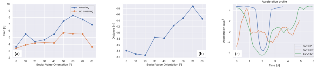
Figure 4.6: (a) Average time to complete the task if the pedestrian is crossing (blue) or if the pedestrian is not crossing (orange). (b) Average minimum distance between the pedestrian and the vehicle. (c) Vehicle acceleration profile with the same episode initial conditions for three SVO values.
